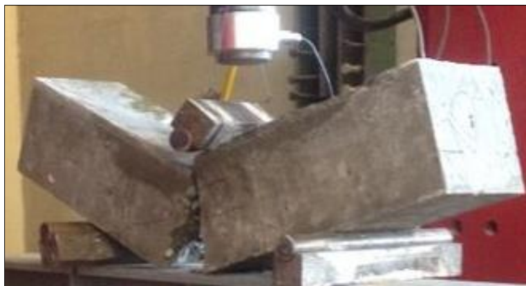
Figure 3: Beam under Flexural Load
