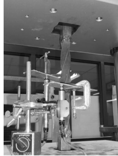
Figure 6: Tensile Testing of a Ransome Bar
