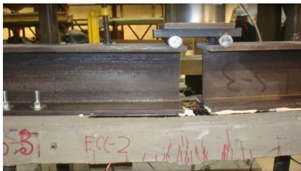
Micro-cracks in LS-ECC
