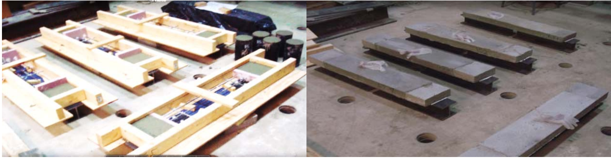
Figure 5: Link slab specimens during casting process and after casting
