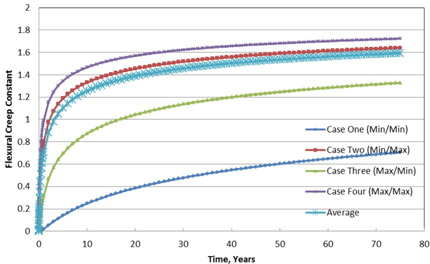
Fig 12: Climate Effect on Long-term Flexural Creep Constant
