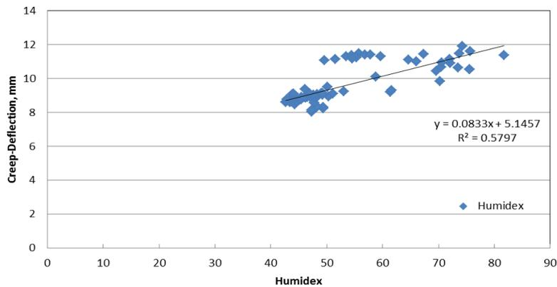
Fig. 8: Effect of Humidex on creep displacement for tested panels BW1, BW2, and BW3
