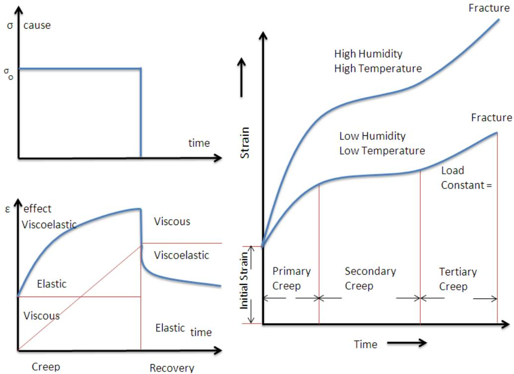
(a) Creep and recovery: Stress,  $\sigma$ , and strain,  $\epsilon$ , vs. time,  $t$  (b) Regions of creep behaviour: Strain,  $\epsilon$ , vs. time,  $t$ , for different Humidex
