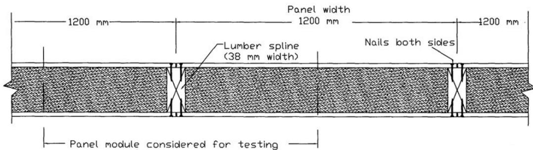
Fig. 2: Typical section at panel lumber-spline connection before and after assembly
