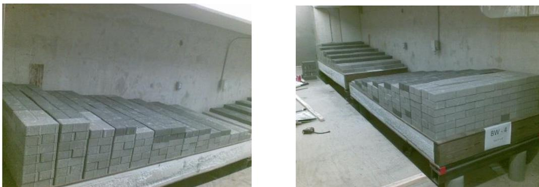
Fig. 3: Views of the simulated triangular loading over the panels
