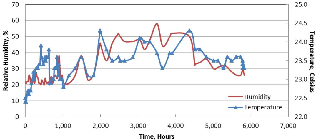
Fig. 4: Recorded temperature and relative humidity with time during creep testing for specimens BW1, BW2, BW4 and BW5
