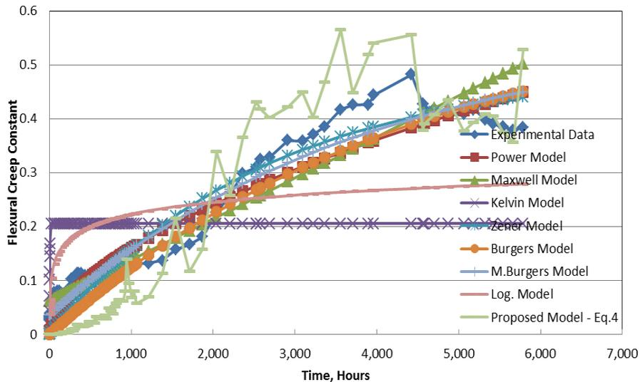
Fig. 10: Measured and predicted Flexural Creep Constant ( $K$ ) versus time for Group I
