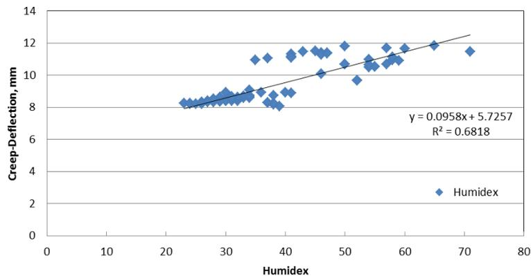
Fig. 9: Effect of Humidex on creep displacement for Tested Panels BW4, BW5, and BW6
