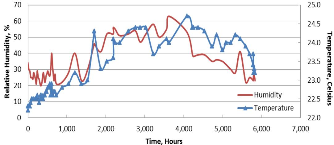
Fig. 5: Recorded temperature and relative humidity with time during creep testing for specimens BW3 and BW6
