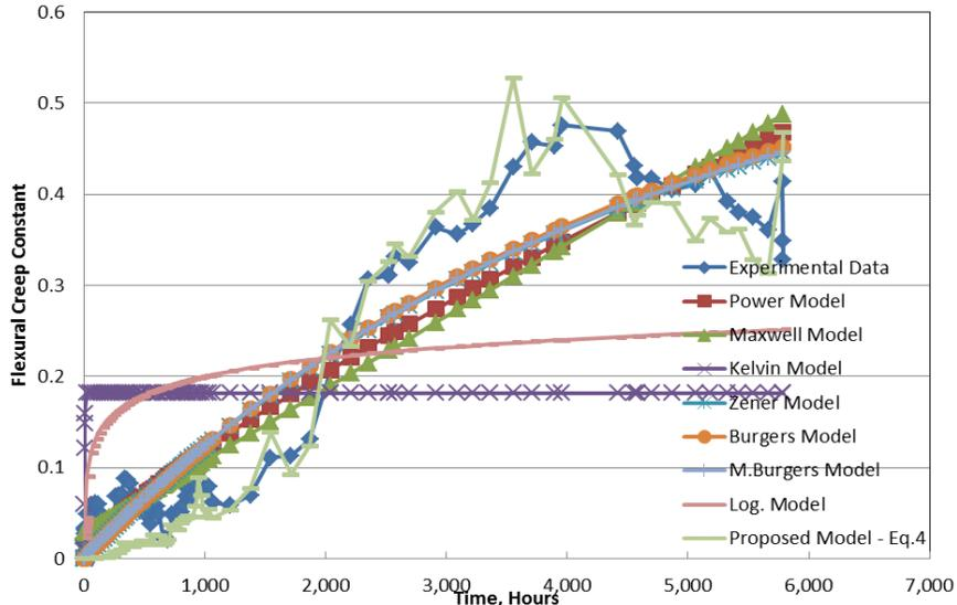
Fig. 11: Measured and predicted Flexural Creep Constant (K) versus time for Group II
