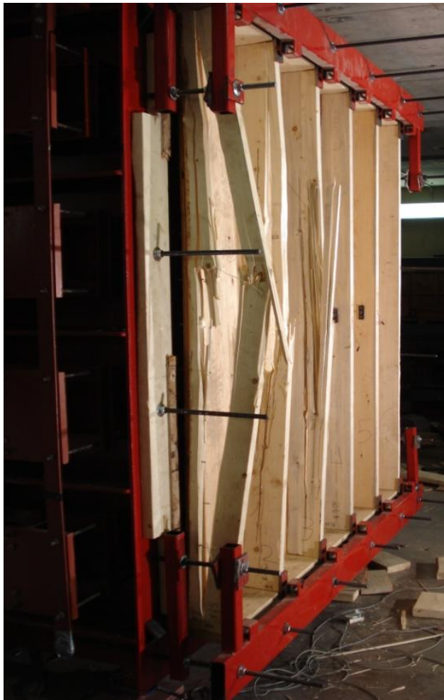
(a) Typical plywood wall after dynamic testing
