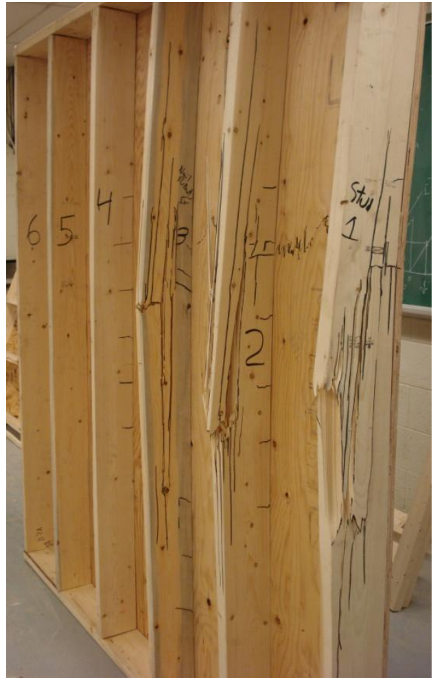
(b) Typical plywood wall after static testing
