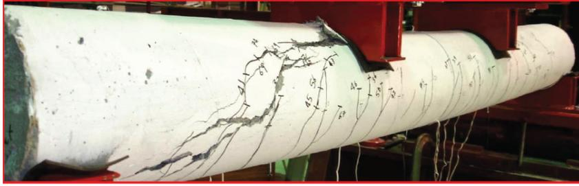
Figure 1. Shear failure mode of FRP-circular concrete beam by Mohamed (2010)
