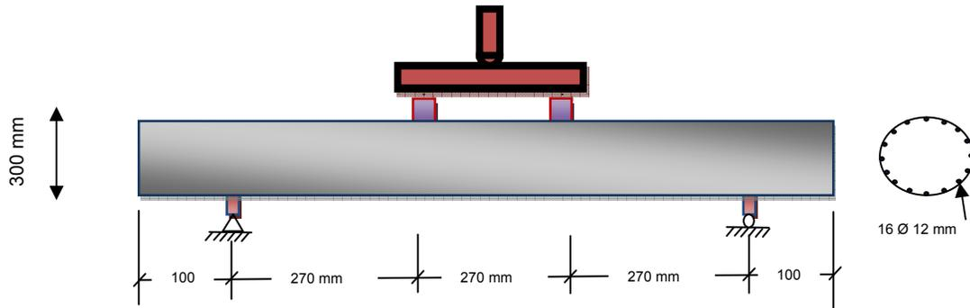
Figure 2. Dimension of FRP beams
