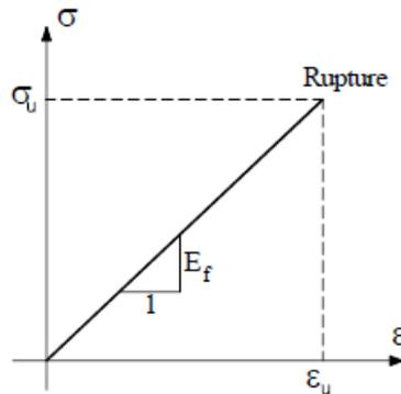
Figure 4. Typical stress–strain relationship for FRP bars
