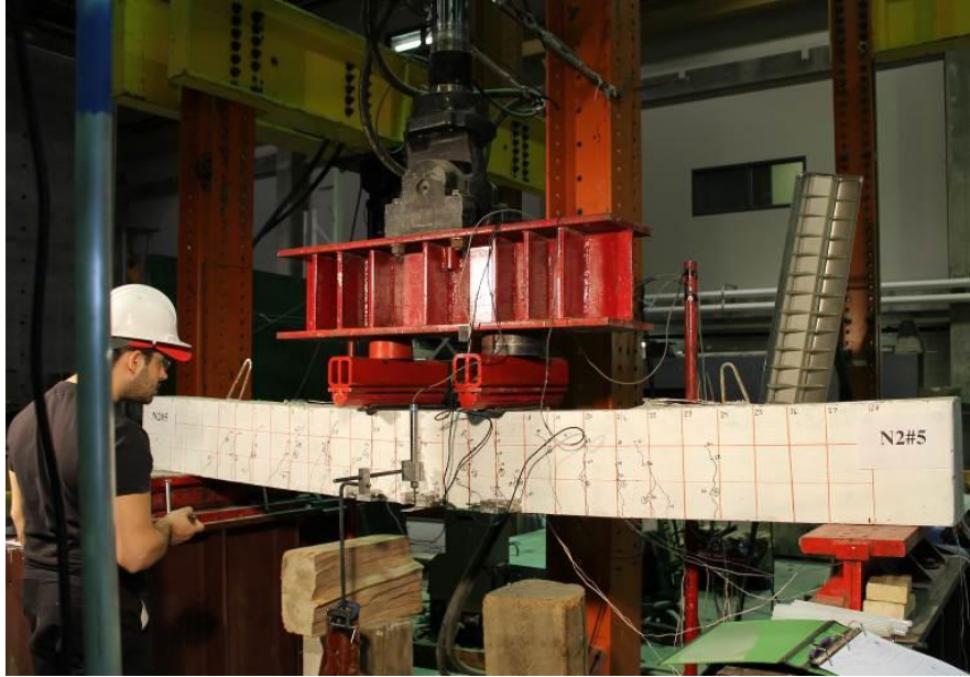
Figure 6: Test setup during a beam test
