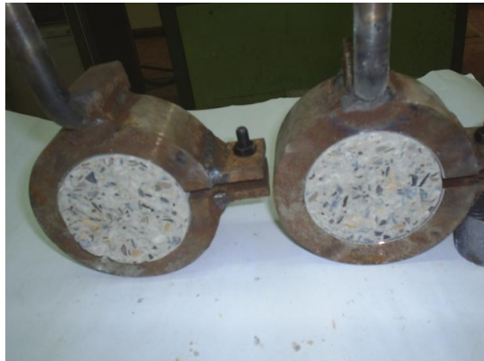
Figure 2: Typical Failure Pattern After Testing
