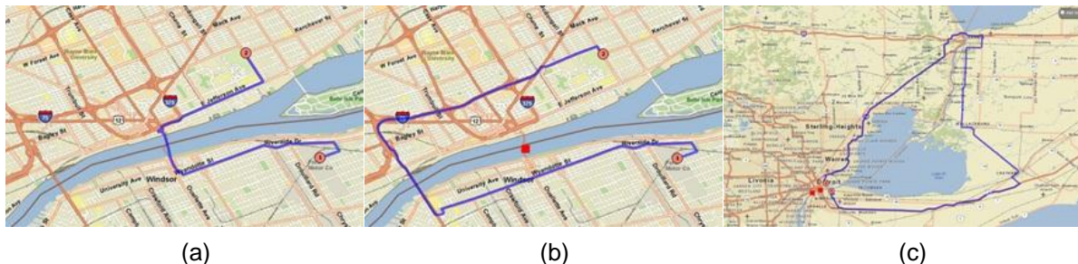
(a) Shortest Route between Detroit and Windsor through the Tunnel, (b) Shortest route after closing the Tunnel through Ambassador Bridge, (c) Shortest Route after Closing the Tunnel and the Bridge
