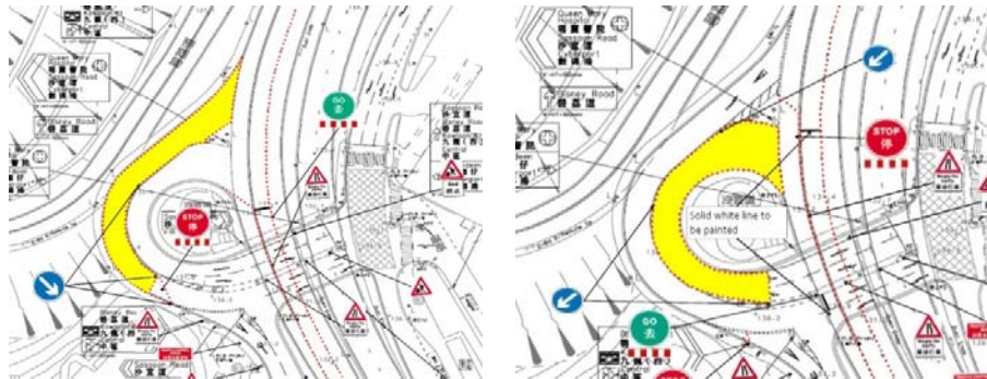
Figure 2: Stage 1 and stage 2 of HMA pavement resurfacing project at Pokfulam Road in Hong Kong
