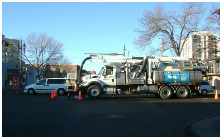
Figure 1: PM vehicle (combo unit) performing high-pressure flushing
