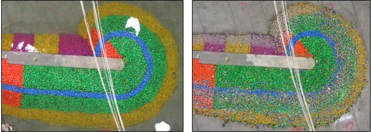
Figure 7. Test series D – overhead view of the 8-12t berm roundhead before (left) and after (right) the testing.
