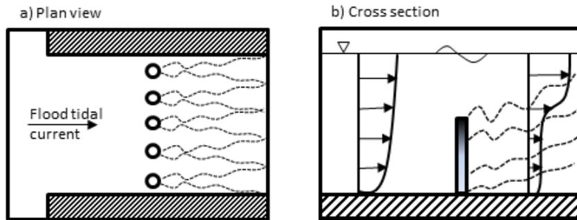
Figure 4: Schematization of turbine implementation, a) plan view of an idealized turbine array across Minas Passage and flow drag added by the structures; b) cross-section showing modification of the velocity profile due to drag added by the bottom-founded porous plate.
